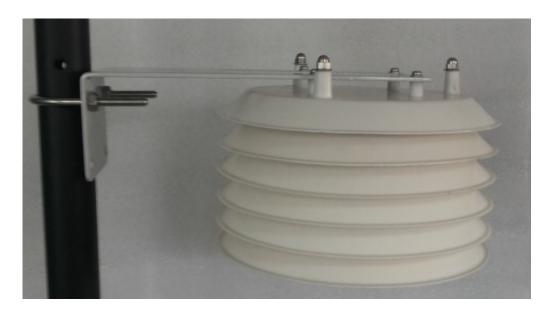
Dust monitor is enclosed in naturally aspirated, 6-plate radiation shield. Its louvered construction allows air to pass freely through the shield, serving to keep the probe at ambient temperature. The shield's white color reflects solar radiation.
