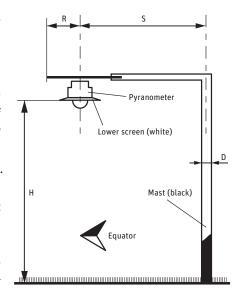
As a guide, a black shadow below the pyranometer with a radius of  $0.1 \, x$  H decreases the signal by 1%, and 99% of the signal will originate from an area with a radius of  $10 \, x$  H.
