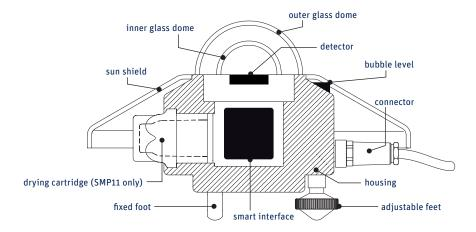
A drying cartridge in the SMP11 radiometer housing is filled with replaceable silica gel and prevents condensation on the inner sides of the domes, which can cool down considerably on clear windless nights. The other SMP's have a sealed construction with a non-replaceable internal drying cartridge. The internal desiccant lasts for 10 years.
