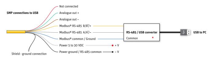
\*Note Switches on the converter should be set for RS-485, 2-wire operation and Echo off.
