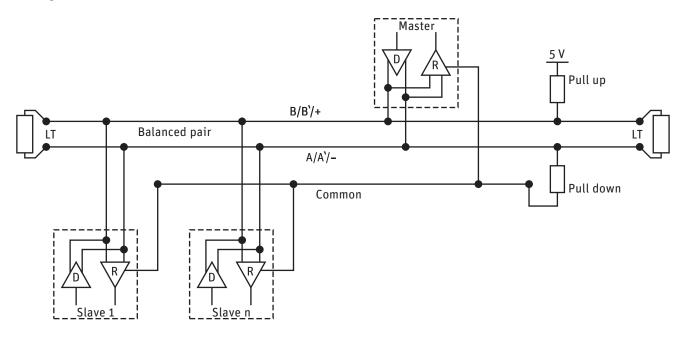
The slaves and master may be a SMP pyranometer or other devices. If a SMP pyranometer is the last device on the network a line terminator (LT), consisting of a 120  $\Omega$  or 150  $\Omega$  resistor, must be connected between terminals A/A'/- and B/B'/+. Never place this line termination on the derivation cable. It is also required to install the pull up and pull down resistors as shown. The value of these resistors must be between 650  $\Omega$  and 850  $\Omega$ .
