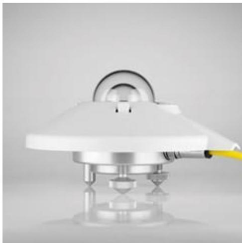
The SMP10 is a spectrally flat Class A pyranometer and has an internal drying cartridge that will last for at least 10 years if the housing is not opened. This minimizes maintenance significantly. With standardized output and connections of every SMP10, exchanging instruments for recalibration is easy.
