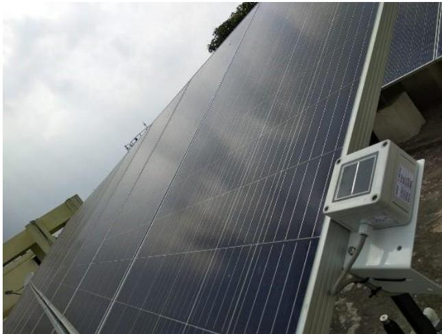
Nes Soz is a low cost Pyranometer with high accuracy and suited for small to medium sized solar projects. The SOZ-03 pyranometer consists of a mono-crystalline silicon cell (50 x 50 mm<sup>2</sup>) with special solar glass. The pyranometer is laminated, hence high UV-resistance and long-term stability.
