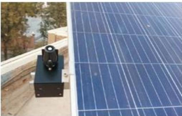
Pyra 300 V is low cost routine/ standard pyranometer suited for small solar project capacity. The sensor's transducer, which converts incident radiation to electrical current, is a silicon photodiode with wide spectral response. From the sensor's output voltage, the console calculates and displays solar irradiance. It also integrates the irradiance values and displays total incident energy over a set period of time.
