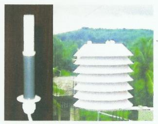
The whole sensor is mounted in a weather shield to protect it from direct solar radiation and rain.
